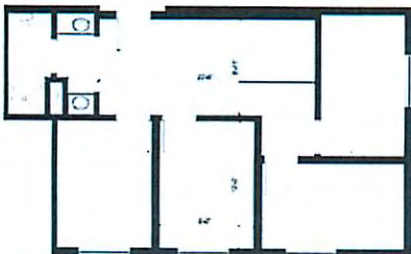
QUAD SINGLES SHARED ROOM 137 SF SINGLE BEDROOM 102 SF SINGLE BEDROOM 102 SF SINGLE BEDROOM 102 SF BATHROOM 78 SF TOTAL 728 SF NET 852 SF GROSS
